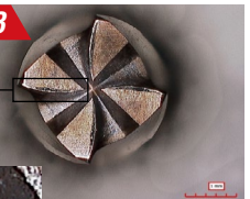
図 荒加工後の摩耗状態 Figure : Wear condition after roughing
