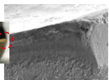
Flute tip after machining 1,000 holes
